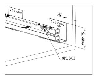
Step 2: Install the basket to the slides connected by fastening.
